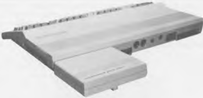
Figure 2-3, RAM expansion module installed
